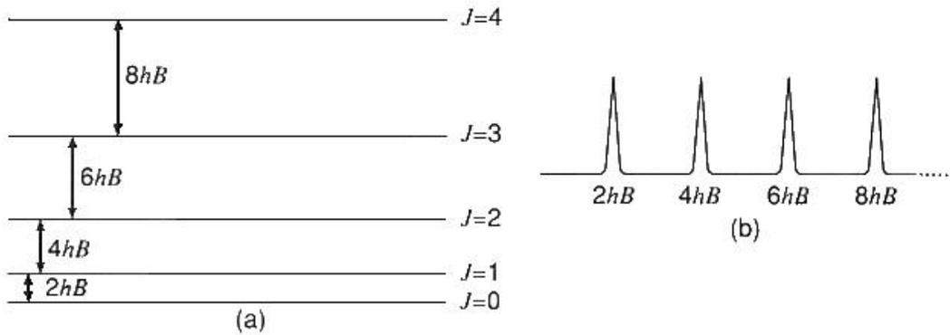
Figure 1.17: The rotational energy levels (a) and the rotational spectrum (b). The rotational constant,  $B = \frac{h}{8\pi^2\mu r^2}$ . The selection rule for rotational transitions,  $\Delta J = \pm 1$ .
