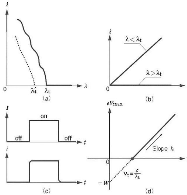
Figure 1.6: Observed features of the photoelectric effect
