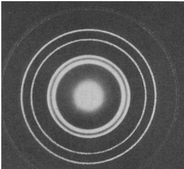
Figure 1.12: Electron diffraction pattern of gold polycrystals
